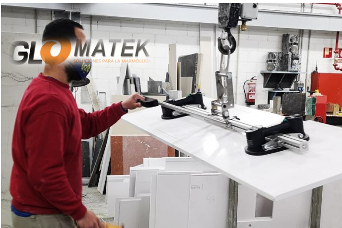
Example of handling with the board horizontal and the handle not locked.
